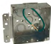
"H" Bracket Narrow bracket allows side-by-side mounting on stud. Positioning tabs locate box perfect distance from stud. V notch centers box. Dimples protect flush drywall installation.
